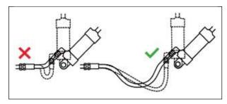
Adequate hose length is most important to distribute movement on flexing applications and to avoid abrasion.
