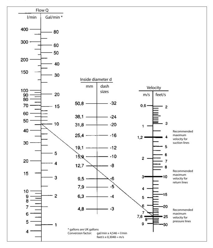
It is therefore important to calculate correctly the required flow line sizes. Undersized pressure lines results in high fluid velocity causing an excessive pressure drop, and heat built up, which impair overall system performance.
