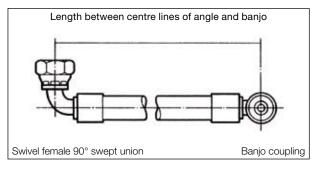
Remember that hydraulic hose under pressure will elongate up to 2% of its length or contract up to 4% depending on pressure, type and size. Sufficient allowance should be made to permit such changes in length.
