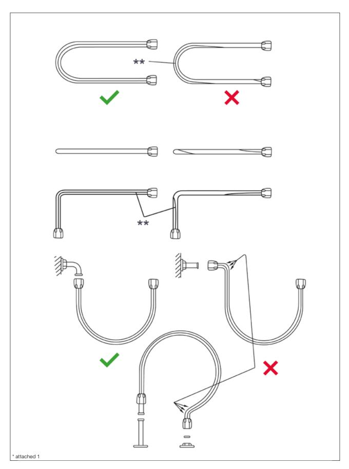
This drawings refer to assemble installed in real conditions. Some of these may request layouts violating such recommendations. It is necessary to point out that such cases are only applicable in test conditions and cannot be used for general use.
