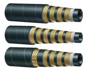
Tube: oil and water resistant synthetic rubber. Reinforcement: four or six high tensile steel spirals or four high tensile steel spiral and one steel braid. Cover: oil, water and ozone resistant synthetic rubber. Application: vey high pressure water jetting. Constant operation: -10 °C +70 °C (14 °F +158 °F) Safety factor: 2,5:1 Length: see below grid.
