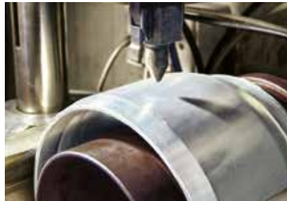
2 Ferrule marking for full traceability
