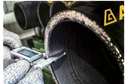
3 Hose thickness measurement is taken to identify the correct calibrated crimping diameter
