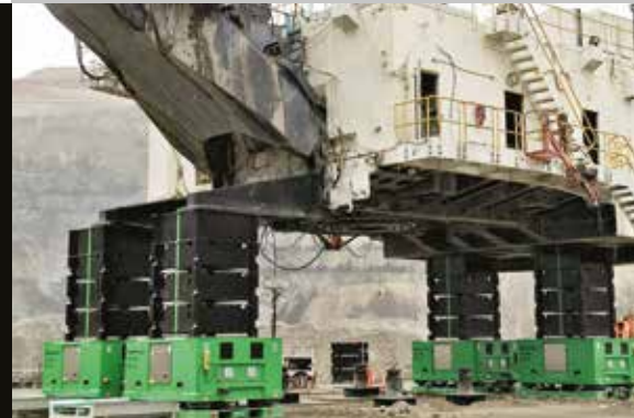
The Enerpac JS500 Jack-Up system has a lifting capacity of 2000 ton.
