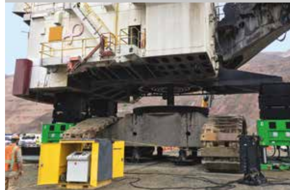
Lifting barrels are stacked together to mechanically hold the load.
