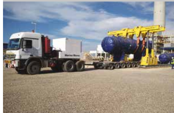
Lifting the high-pressure heater off the transport trailer.
