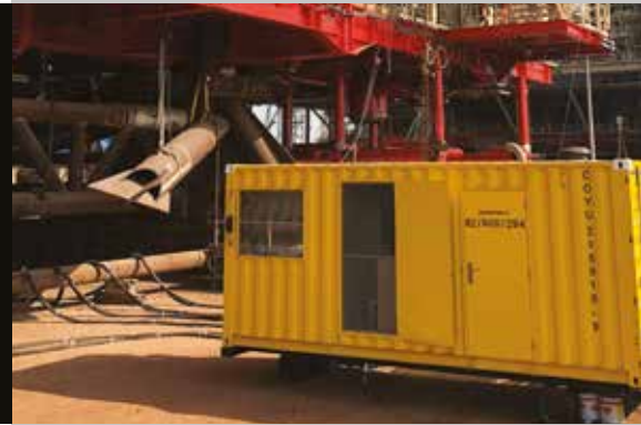
Enerpac Self-Propelled Power Pack that powered the 'Push-Pull' system for the platform load-out.
